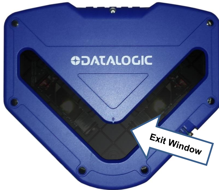
Figure 79: Exit window locations
